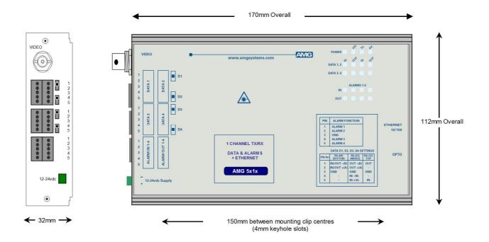
The **AMG5918** is a standalone one channel video receive unit designed to receive 1 video signal and transmit and receive 4 data signals plus 4 bi-directional alarms and also provides full duplex 100Base-T Ethernet connectivity over one Singlemode optical fibre.
